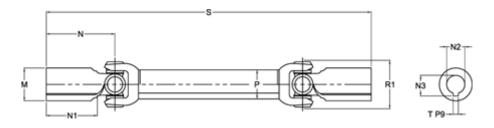
S min = 534Μ = 90 Max. Bending Angle degrees = 35 = 16 Ν = 175 = 87 N1 = 55 H7 N2 = 59,3 +0,2N3 Ρ = 70x4R1 = 125
